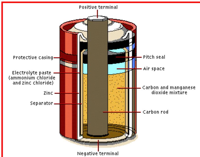
The functional elements of a dry cell battery are the negative terminal (a zinc can which encloses the battery materials), the positive terminal (the carbon rod and carbon and manganese dioxide mixture that surrounds the rod), and an electrolyte paste between the two terminals. The electrolytic paste facilitates a chemical reaction involving the constituents of both terminals; this reaction causes a current to flow through a conductor that connects the positive and negative terminals.
